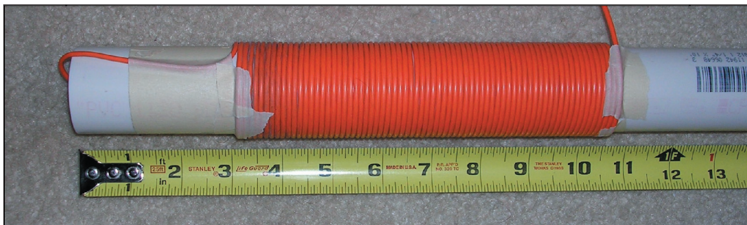
The first layer is complete and its ends are secured with masking tape. Note the extra wire that is tucked into the left end of the PVC pipe.
