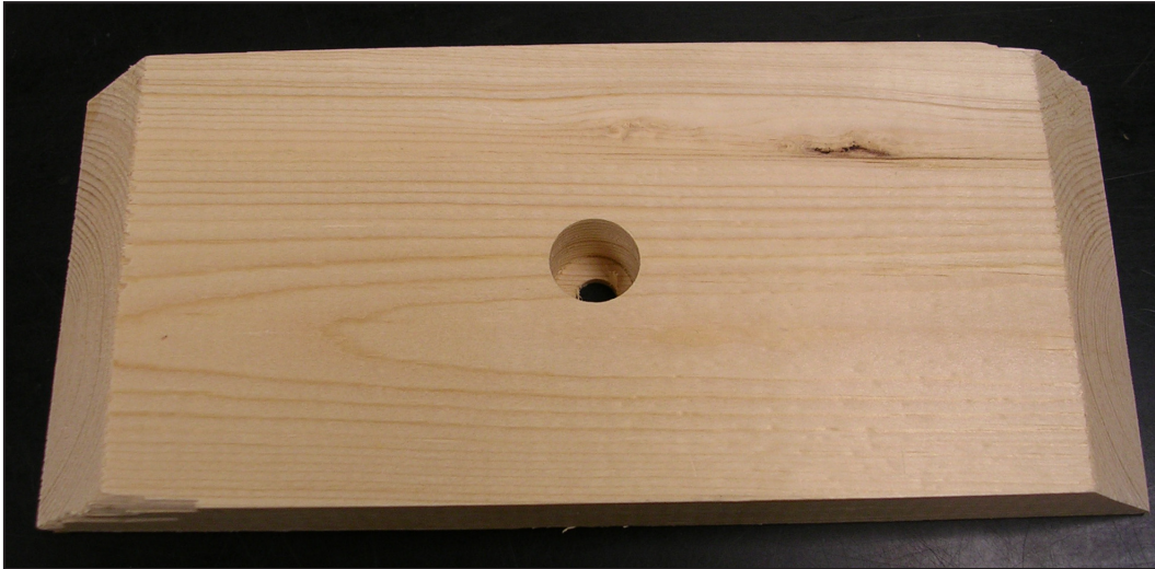
The base's back board had been cut and a hole for the power jack has been drilled through it.
