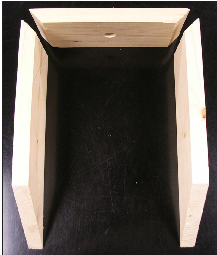
The three sections of the base, prior to joining, showing the correct miter cuts.
