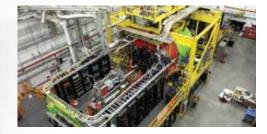
Hall D is configured with a superconducting solenoid magnet and associated detector systems that are used to study the strong force that binds quarks together.
