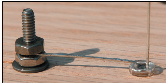
Trapping the cathode between a pair of hex nuts can save some soldering!
