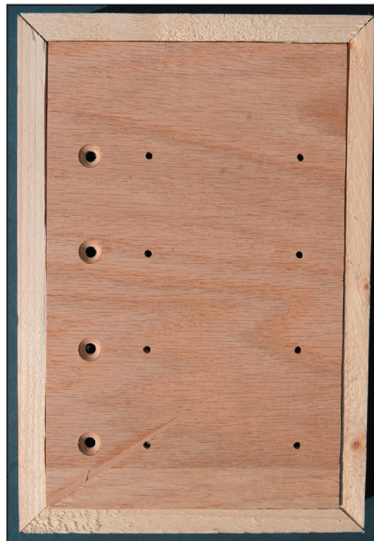
The plywood panel has been glued to the base.
