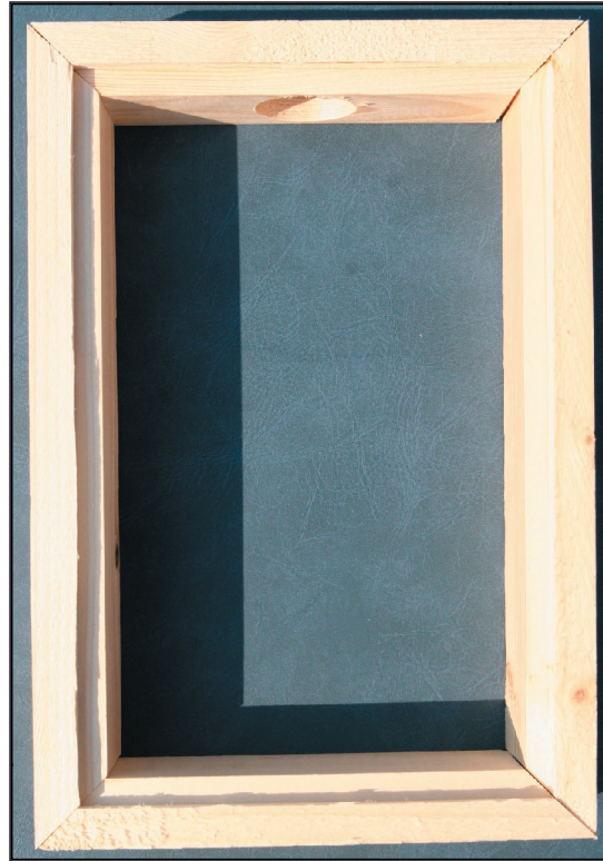
The base pieces have been joined together.
