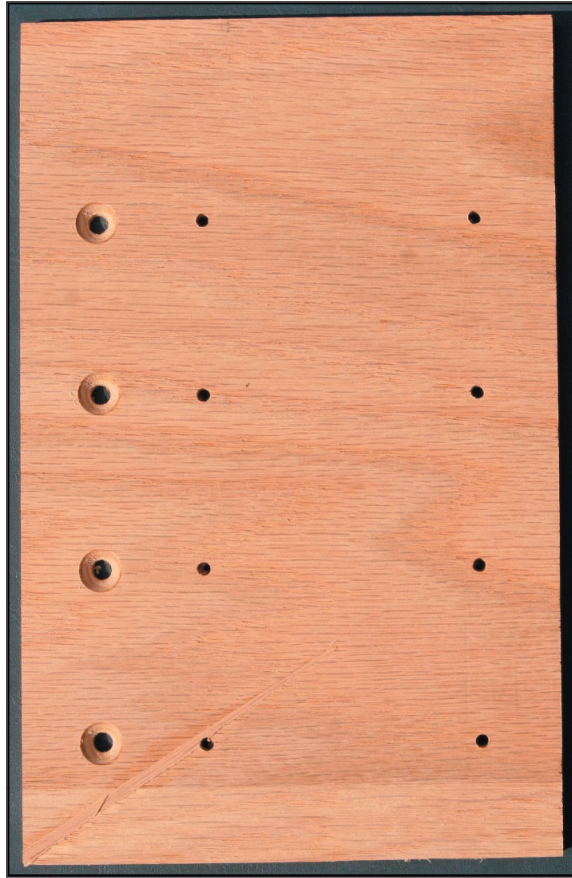
Holes for the LEDs and fuse clips have been drilled in the plywood panel.
