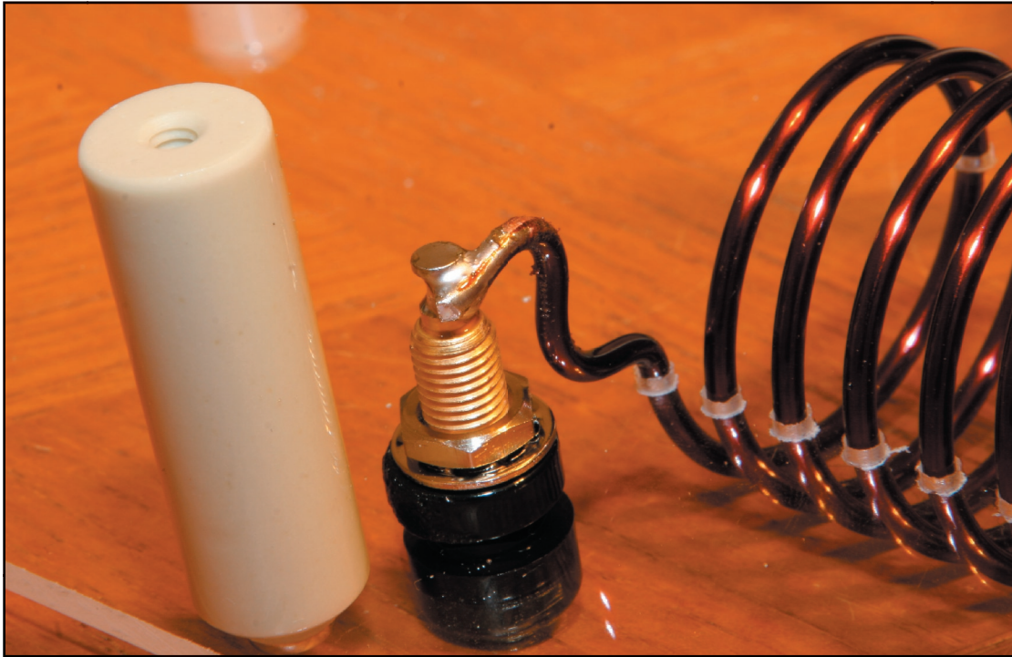
The coil's leading end has been soldered to the banana plug panel mount's soldering post.
