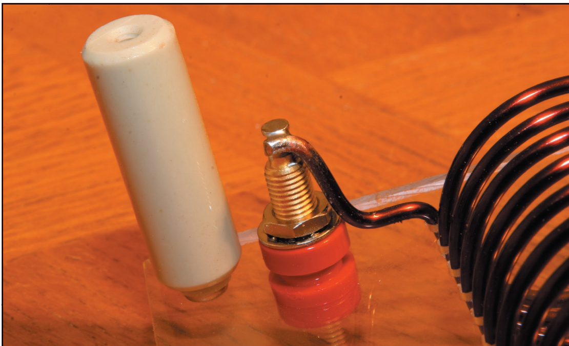
The coil's trailing end has been soldered to the banana plug panel mount's soldering post.
