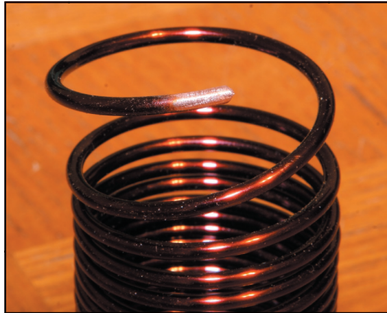
The insulation has been removed from a section of the coil.
