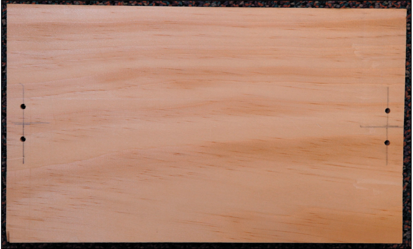
Pilot holes have been drilled in the base board.
