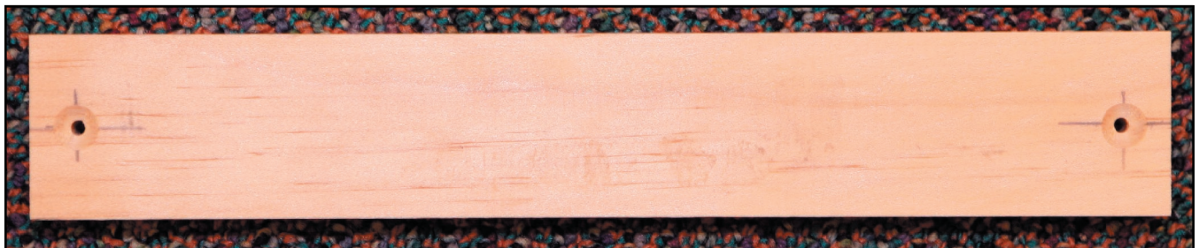
Pilot holes have been drilled in the top board.
